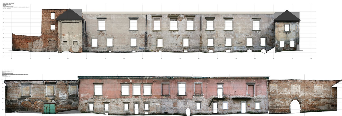
Fig. 3. Orthogonal photogrammetries of the Palace building facades
