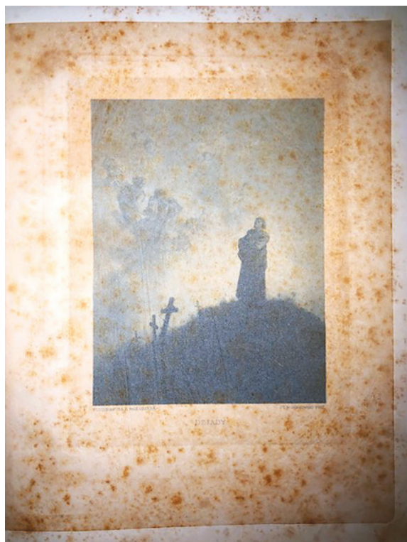
Fig. 7. Various types of foxing spots. Document from the Archives of the Resurrectionist Fathers in Rome.
